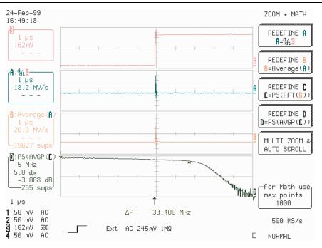
Figure 1 – Transforming the measured step response of a filter into the frequency response.
